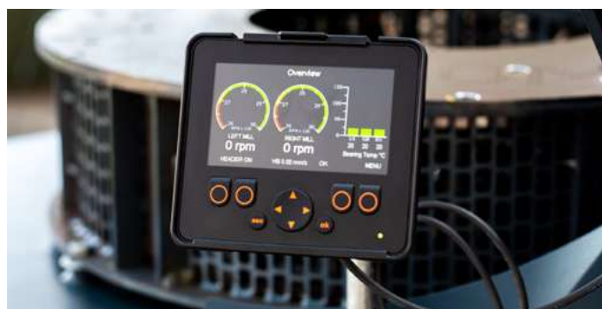
Mill speeds, bearing and gearbox temperatures, vibration and blockage sensors are visualised in the operator terminal.
