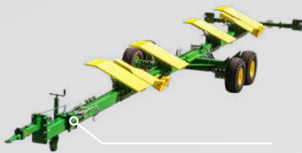
SWW 400 Tandem-axle header transporter
