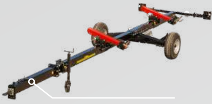
SWW 100 | 200 | 300 Single-axle header transporter
