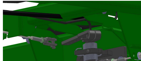
Disconnect the cables from the transfer lever when setting up the wheel brakes.
