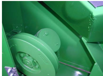
Lubricate the knife bar drive (5 squirts of the grease gun every 50 operating hours)
