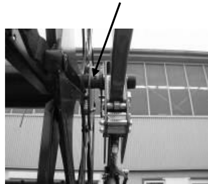
(both sides) Lubricate body of reel shaft (5 strokes of grease gun or until grease is escaping )
