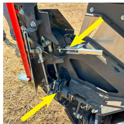
The side knives are simply latched into place, and the drivelines are connected by coupling a dog clutch. Changeover is a 5min job.
