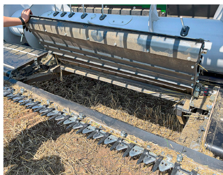
The belts simply fold up and out of the way for maintenance – much easier for the operator.
