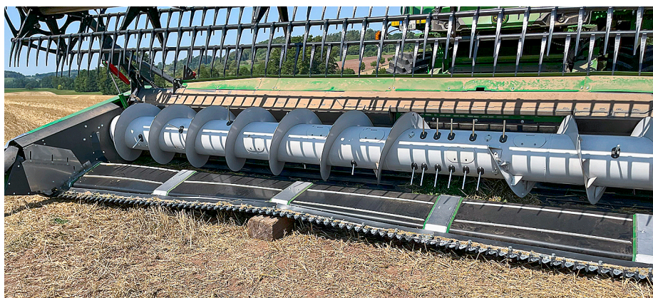
The cutterbar is able to flex by up to 15cm.
